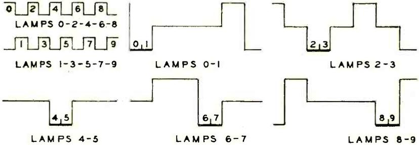
Fig. 7—Derivation of indications in binary decade.
