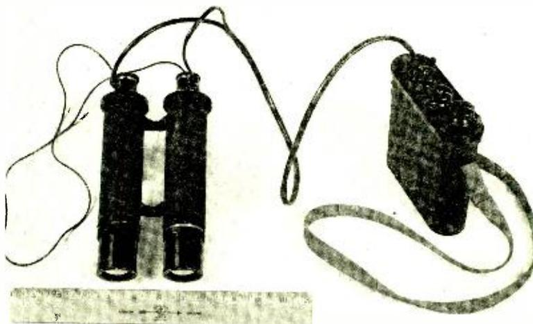
Fig. 10—Infrared In-line Binocular.
