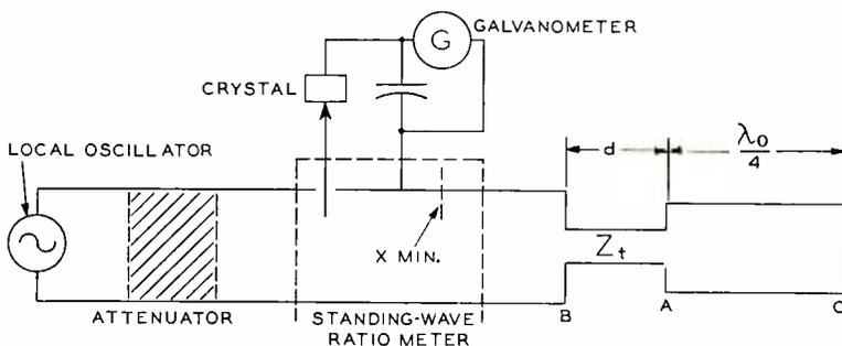
Fig. 3—Experimental setup for determining transformer "end-effects".
