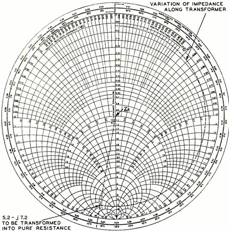
Fig. 5—Determination of correct transformer length.
