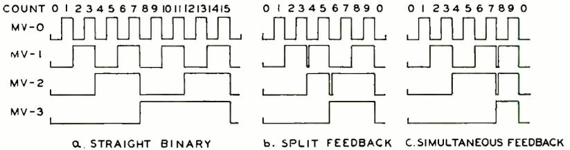
Fig. 5—Application of feedback to binary chains.
