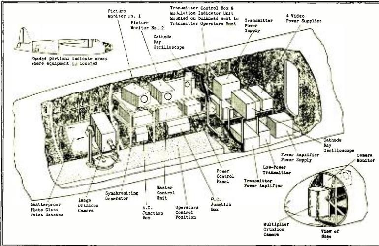
Fig. 17—Phantom view of the location of the various units in the JM-1 aircraft. The transmitter is located in the after bomb bay, and the antenna is located just forward of the transmitter beneath the fuselage.
