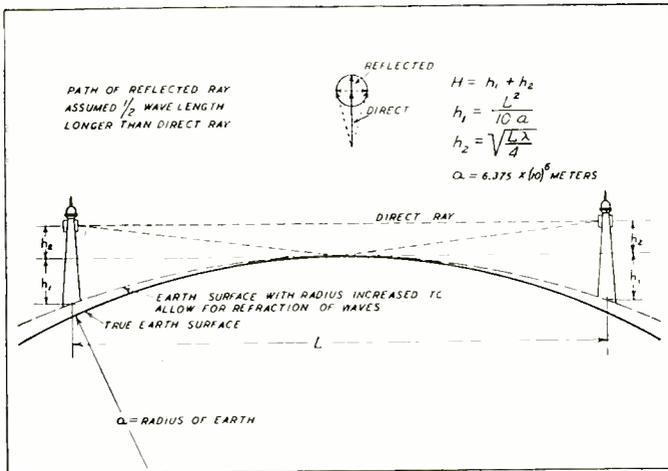
Fig. 3—The radio relay space circuit.
