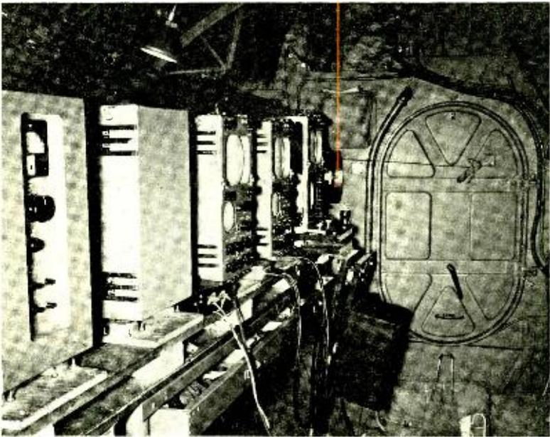
Fig. 1—Control position in PBY-4 aircraft installation using commercial television equipment.
