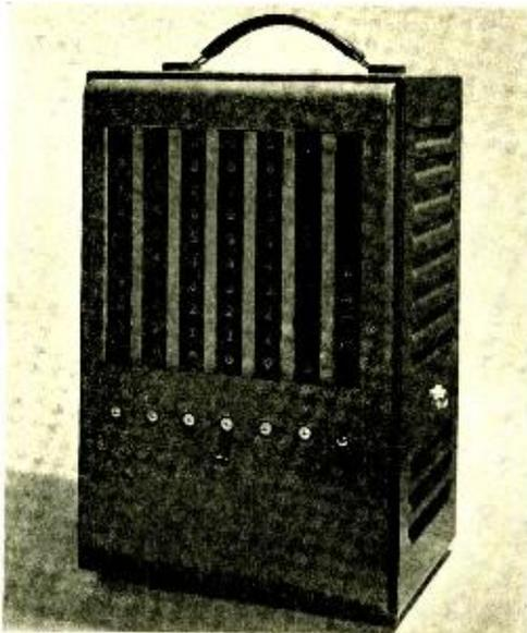
Fig. 14—A current model of the electronic counter.
