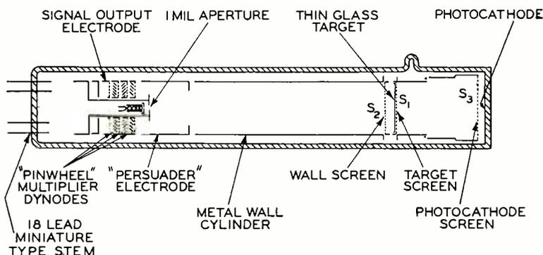
Fig. 3—Cross-sectional diagram of the Mimo tube.
