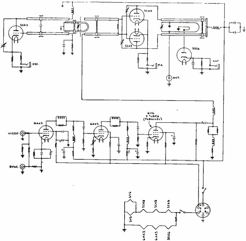
Fig. 7—Mimo transmitter diagram.
