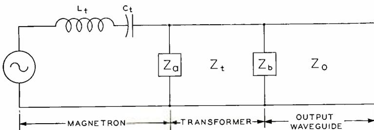
Fig. 2—Schematic diagram of waveguide-output magnetron.
