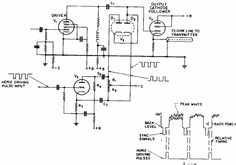
Fig. 9—Keyed black-level clamp circuit.
