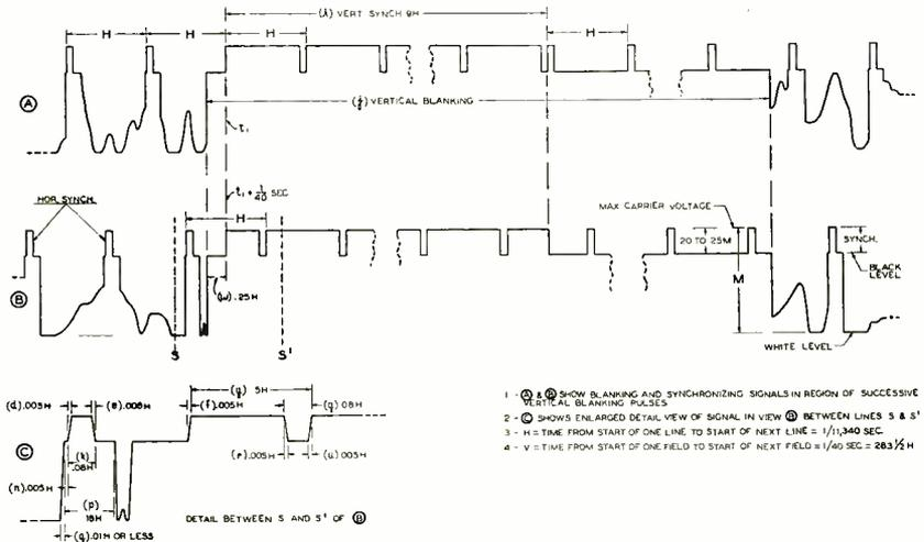
Fig. 5—Synchronizing signal waveform used for Project Ring.
