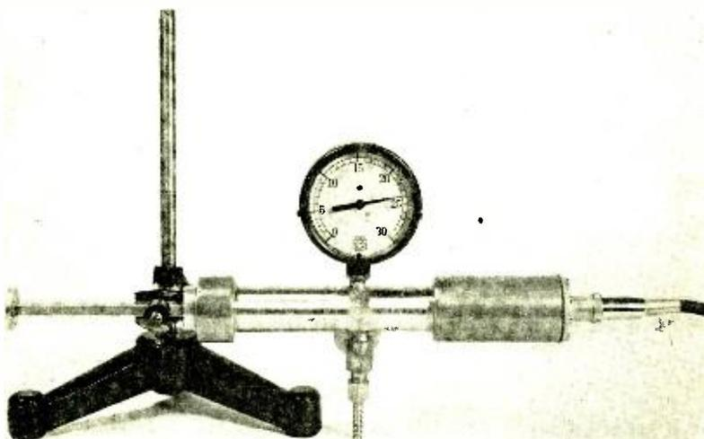
Fig. 4—Photograph of resonant receiver.
