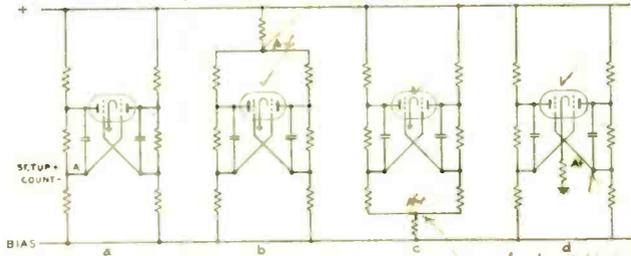
Fig. 1—Resistance coupled multivibrators.
