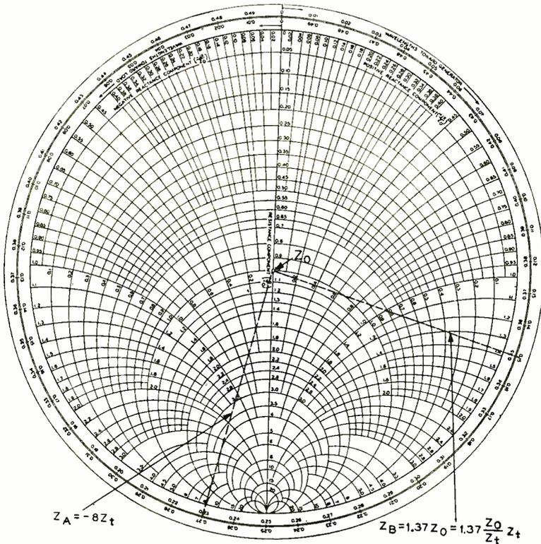
Fig. 4—Transformer "end-effect" reactances.
